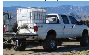
Pick-up Trucks with IBC Tote & Pumps
